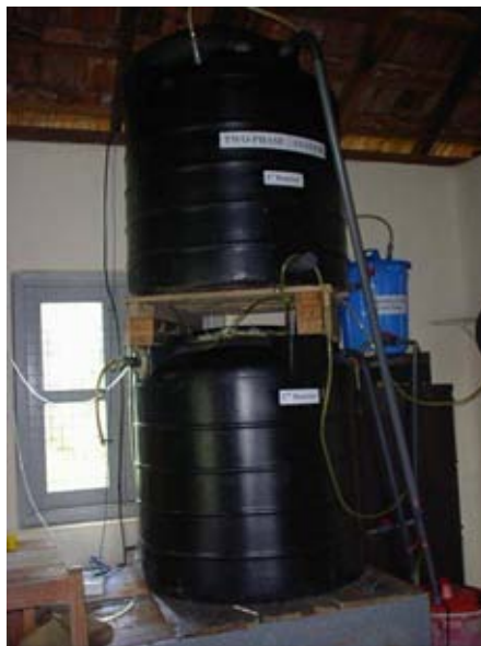
Fig. 4: Designed and fabricated two-phase reactor system
